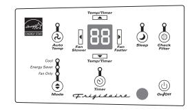
A 2 Digit Display is used to indicate the Fan Speed setting, from 10 through 99. When the "SLOWER" button is pressed the motor speed will slow down at various intervals, down to a minimum setting of 10. To speed the motor up, press the "FASTER" button. The speed will increase at multiple intervals to a maximum setting of 99. Display will revert back to temperature setting after a short time.
